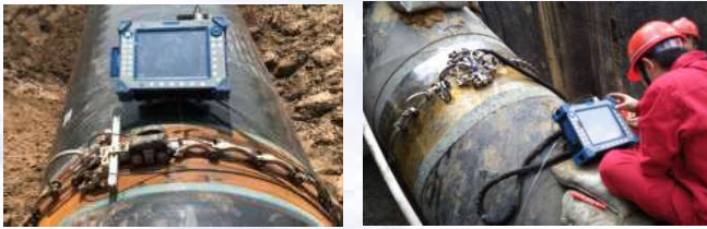
Fillet Weld Inspection of Socket (Real-time Update of Weld Cross Section)
