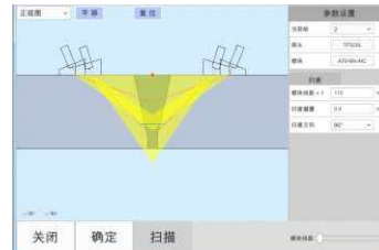
TOFD Beam Coverage Simulation
