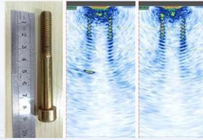
TFM Inspection of Small Screw
