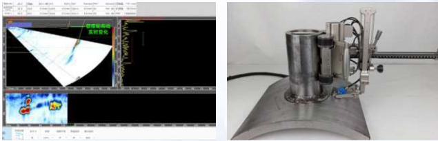
Fillet Weld Inspection of Socket (Real-time Update of Weld Cross Section)
